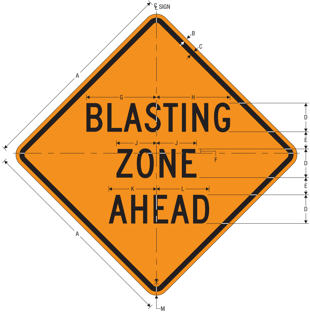
W22-1 BLASTING ZONE AHEAD
