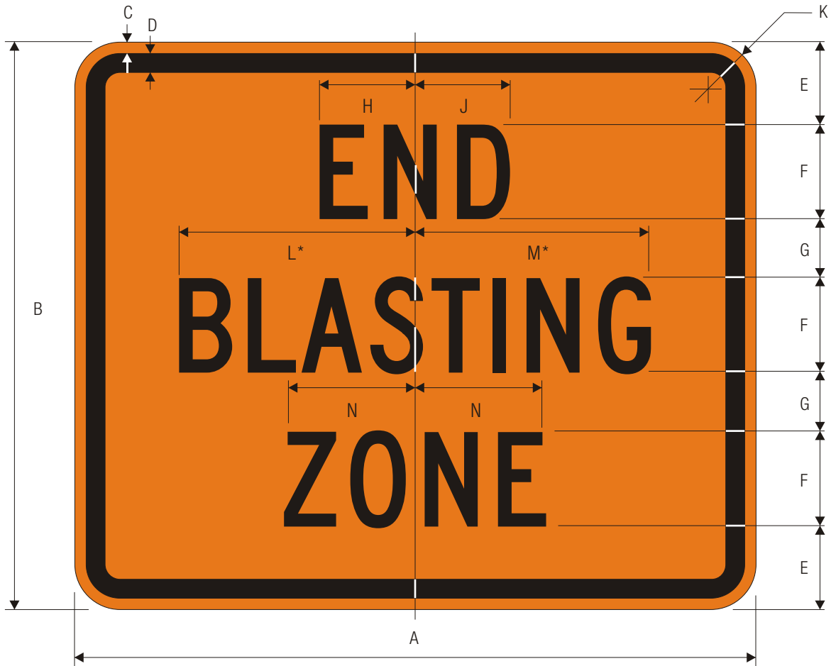
W22-3 END BLASTING ZONE
