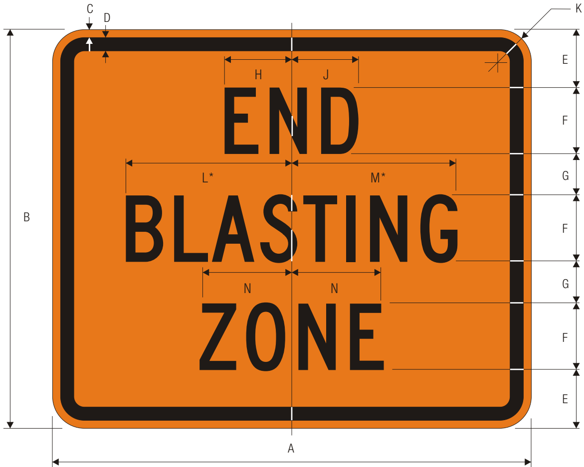
W22-3 END BLASTING ZONE
