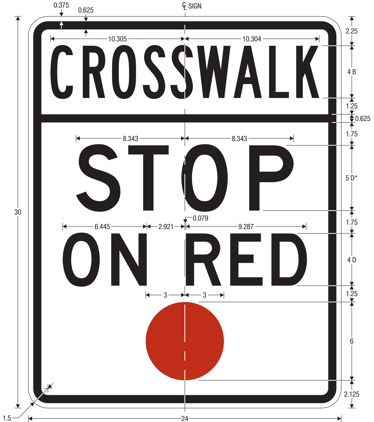
R10-23 CROSSWALK - STOP ON RED
