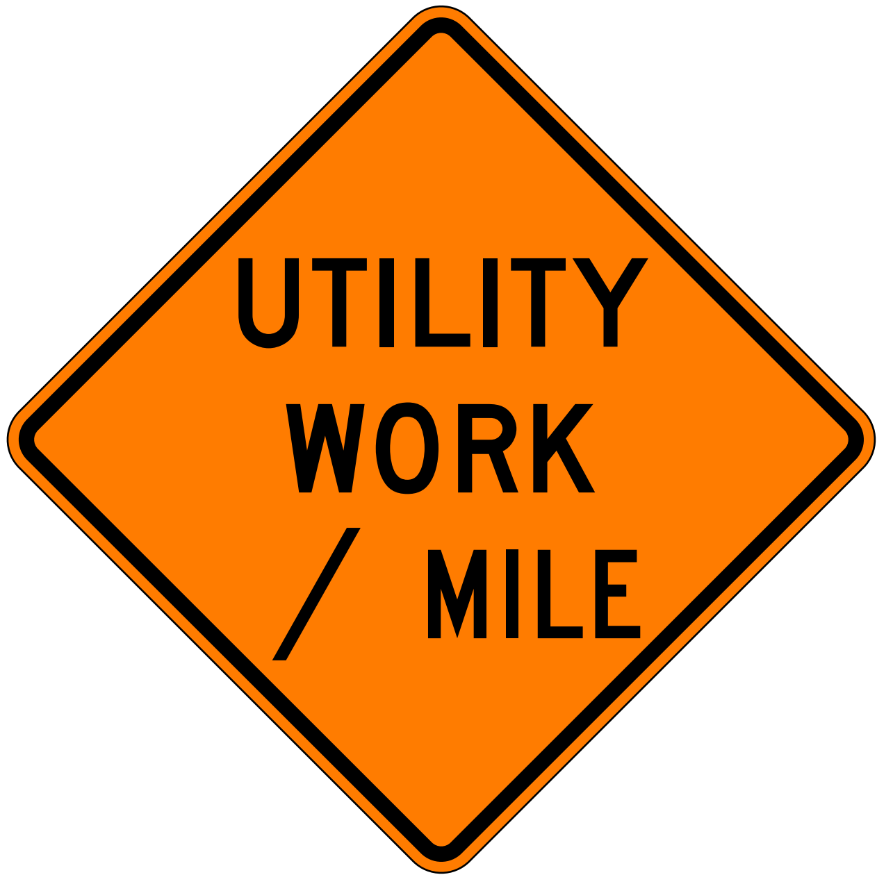
W21-7 Utility Work (Distance)
