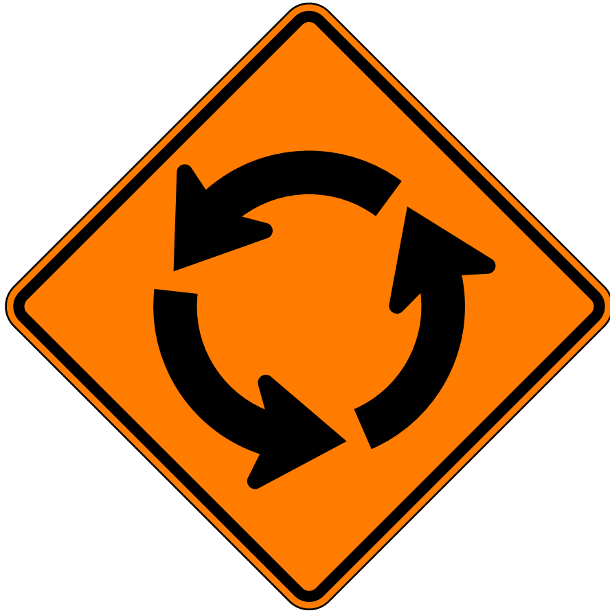
W2-6 Roundabout Intersection
