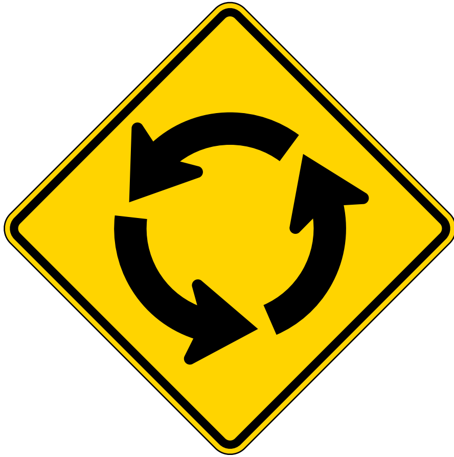
W2-6 Roundabout Intersection
