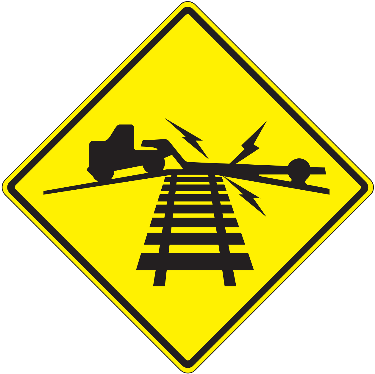
W10-5 Low Ground Clearance Railroad Crossing
