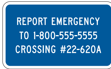
Figure 8B-5. Example of Emergency Notification Sign
